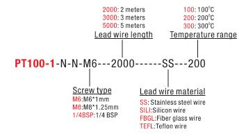
This is a most commonly used screw-in type PT100, standard version with M6 screw and 2 meters stainless steel cable
